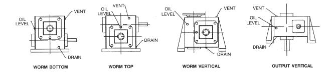
Figure 8 Standard Oil Levels
