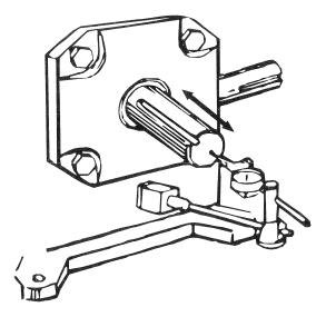
Figure 5 Checking Axial Float
