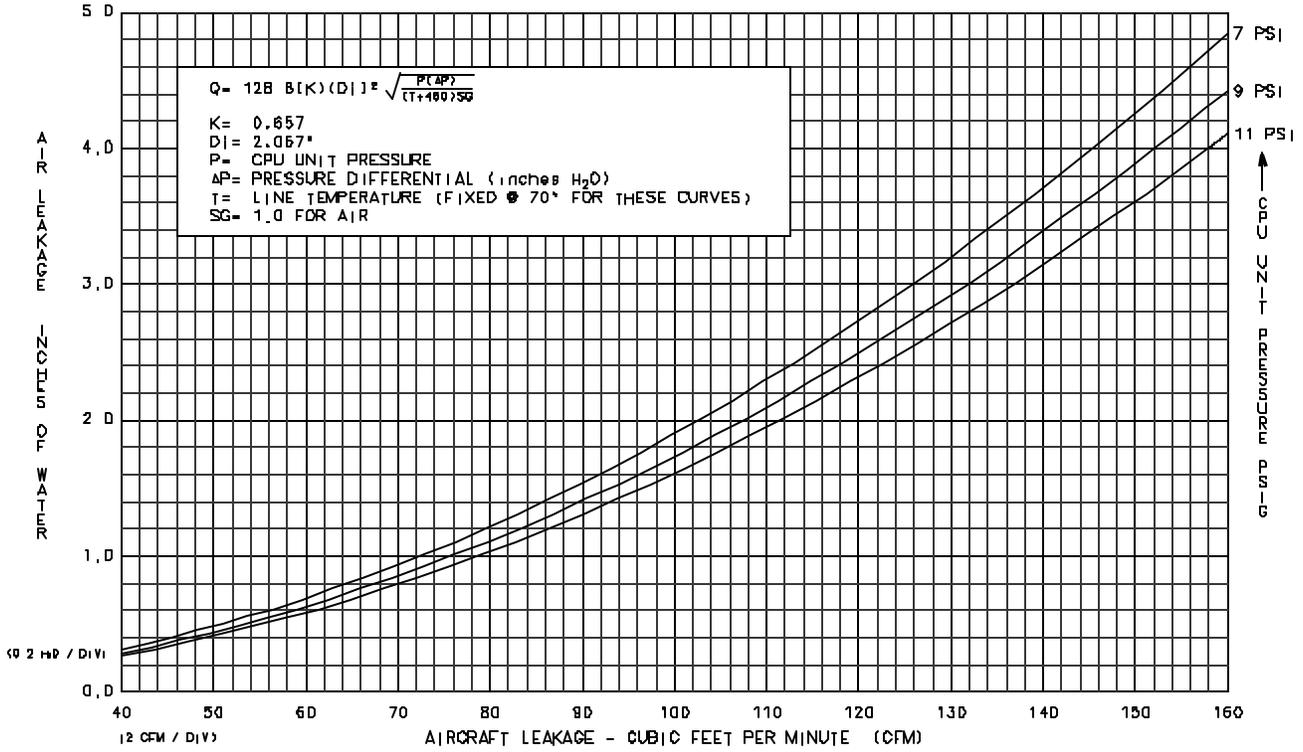
**CURVE #4 TEMPERATURE CORRECTION - DESIGN FLOW TEMP = 70° F**
