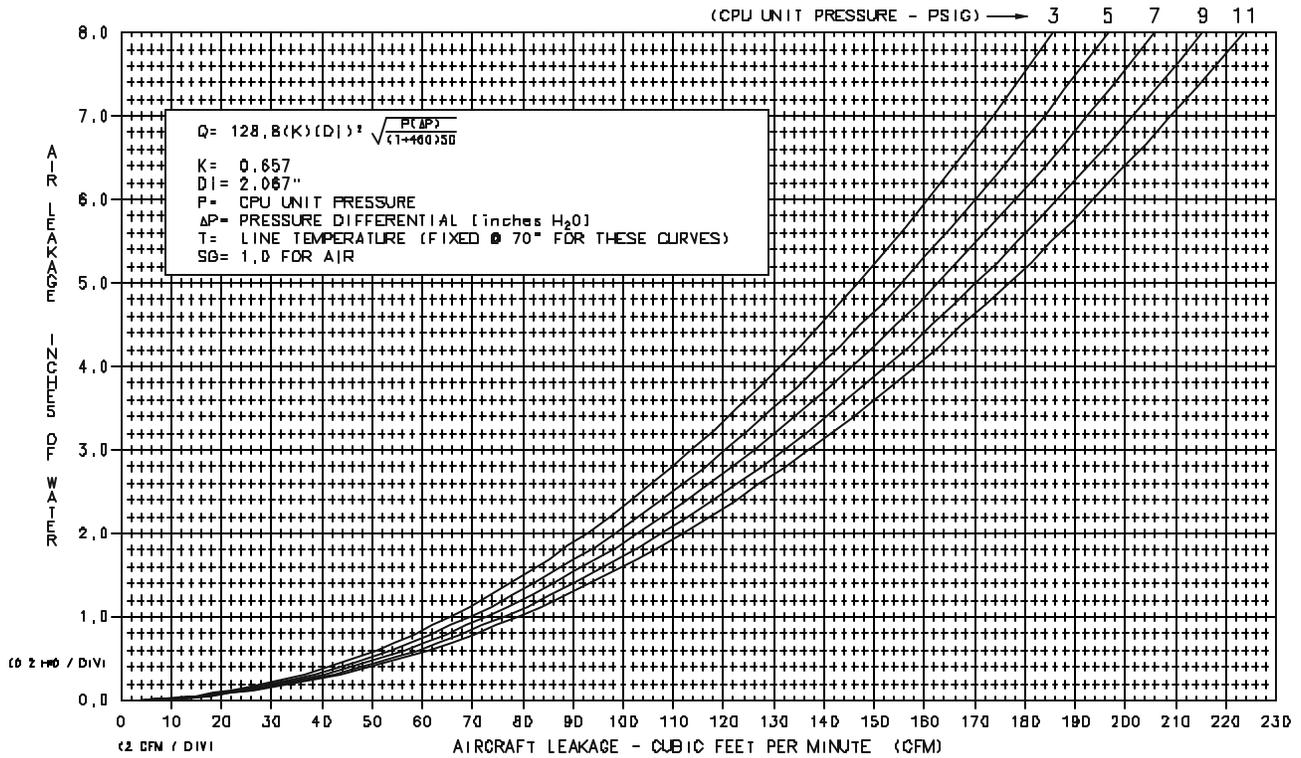
**CURVE #2 PRESSURE COMPENSATED FLOW @ 70° F: INCHES OF H<sub>2</sub>O vs. LEAKAGE**
