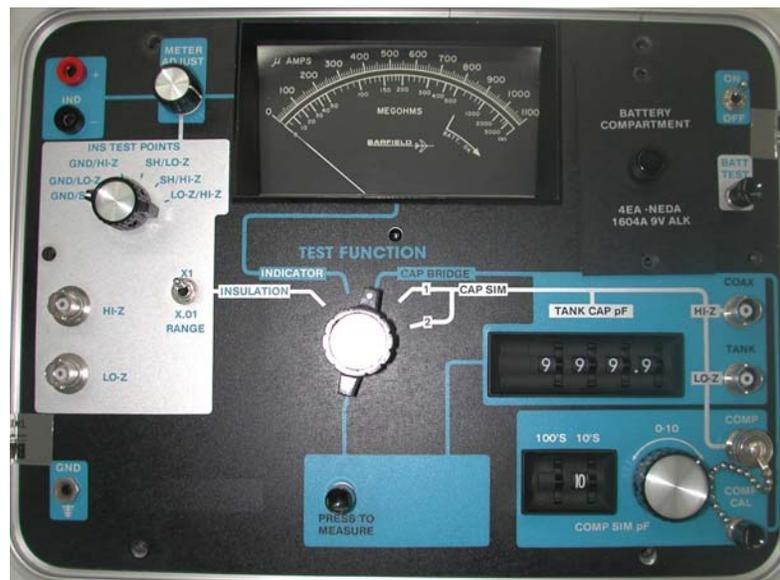
**Figure 4 2548H FUEL QUANTITY TEST SET**
