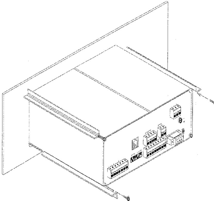
Figure 2-2. Panel Mounting Arrangement
