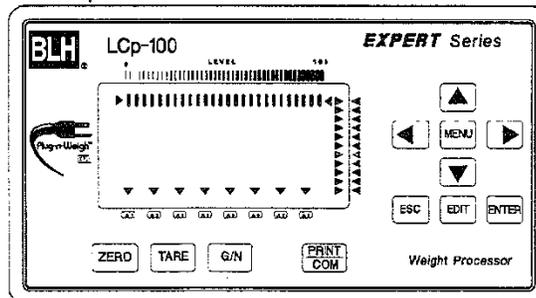
Figure 1-2. The LCp-100 Front Panel
