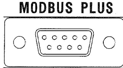
Figure 2-14. 9-Socket Modbus Plus Connector
