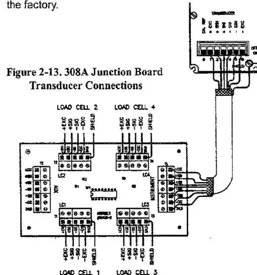
Figure 2-13. 308A Junction Board Transducer Connections
