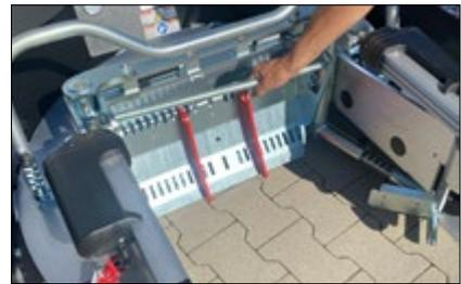
Set the bar for the wheels diameter to fit
