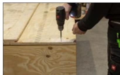
The upper bolts on the side of the front access ramp must also be removed in order to lift the cover.
