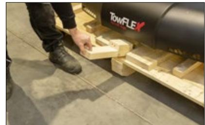
Take the top cover and attach it to the front of the transport box to use it as ramp for the tug.
