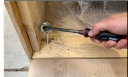
To prevent unwanted movement during transport, there is a wooden wedge in front of the castor wheels, which is bolted to the floor of the box. Remove these bolts and pull out the wedge.
