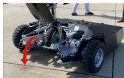
After that, the nose wheel should be cleared and the tug can be moved away from the nosegear carefully.
