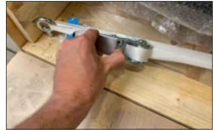
also remove the eyebolts to which the tension straps are attached.
