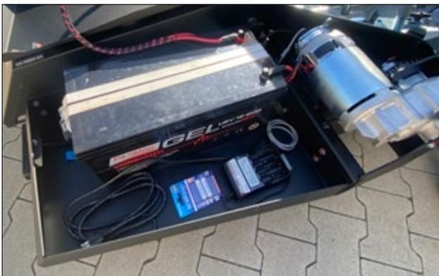
Charger for Tug and Battery Charger for RC Batteries
