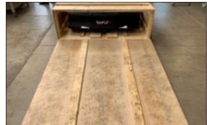
Then pull the two eStops and start the unit. Wait until the unit has booted and the connection has been established. Then you can drive the tug very carefully and as slowly as possible over the ramp.
