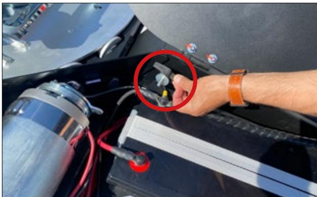
Wing nuts on both sides must be removed
