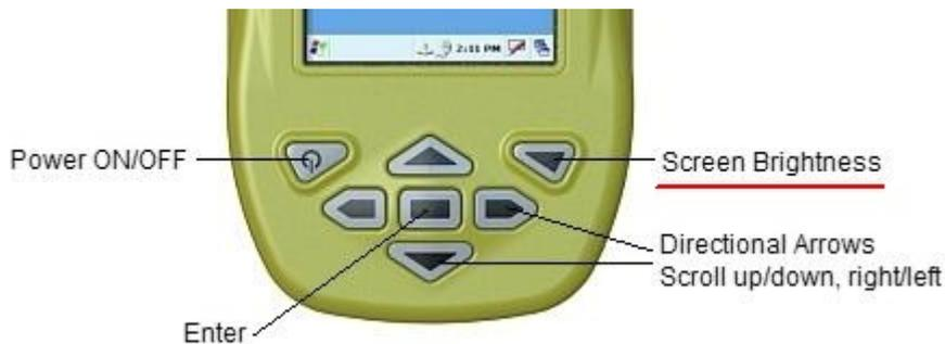
Figure 2-5 *MEZ1500 Keypad - Screen Brightness Button.*
